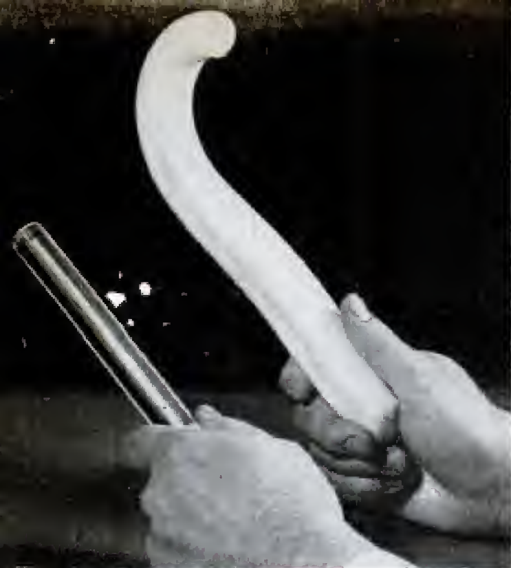
Irradiation-produced gases in a plastic bar cause it to expand when heated, while the same heat has no effect on an untreated bar of the same material
